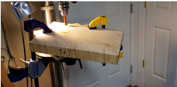
Angle plate for drilling angled mortises by Lou Mansur.
