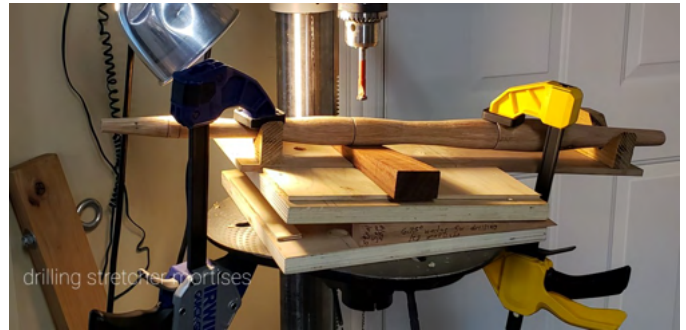
Angle plate for drilling angled mortises by Lou Mansur.
