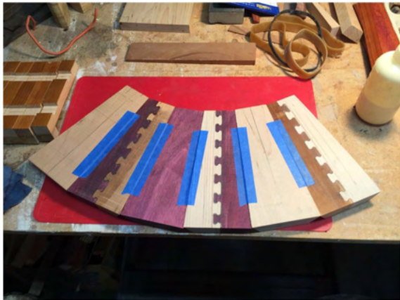
Clamping and gluing fixture for tapered staves by Brian Horais.
