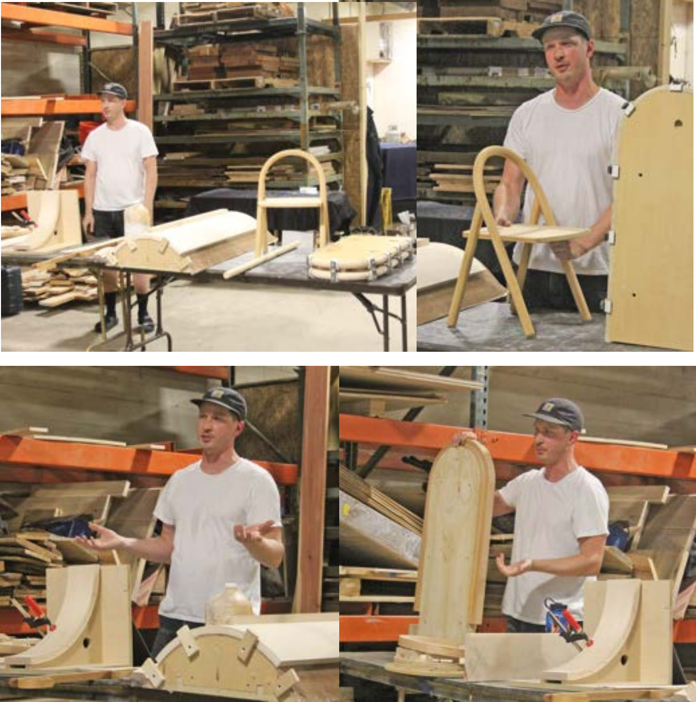
Frank demonstrating different bending forms and processes used in producing his chairs and tables.
