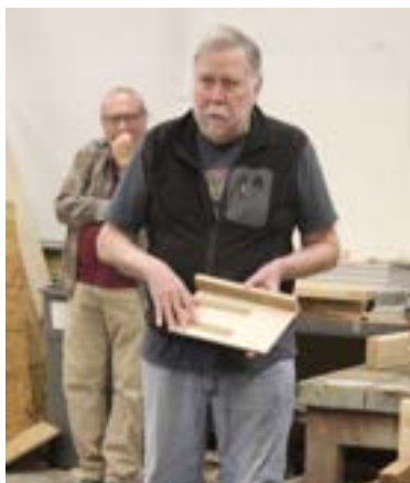
Jig for sawing dovetail tails on the bandsaw.
