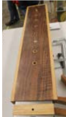
Bench top bench to elevate working height for some task specific that requires a higher bench top, also being portable is a feature, by Stephen Paddison.
