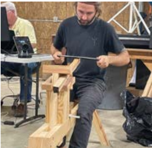
Shaping wood with draw knife utilizing a shave horse to hold the piece being shaped.
