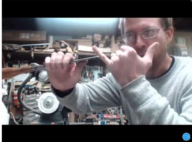
Stephen demonstrated how he sharpens a chisel and uses diamond plates to quickly gain back a workable edge.
